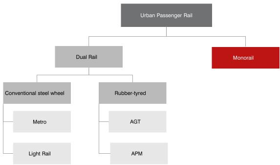
Figure 1: Common urban passenger rail applications
